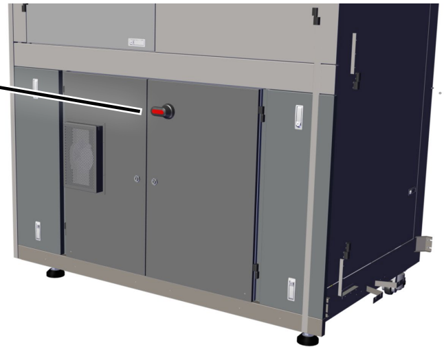
Main Power Disconnect
